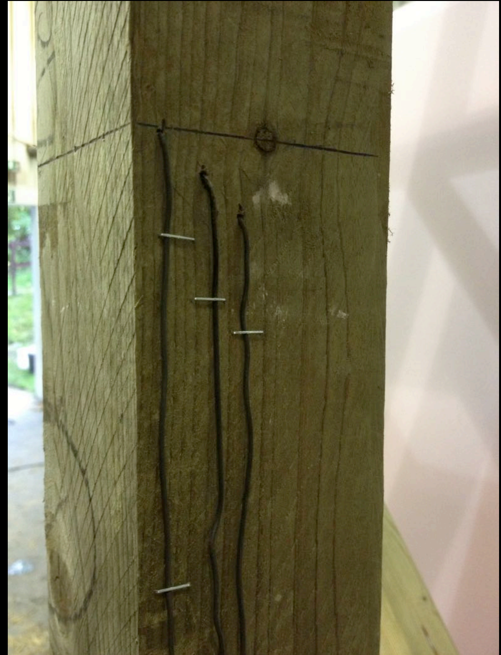
Placing of heat sensors on the posts, the faces of which were set back from the exposed face by 175mm
