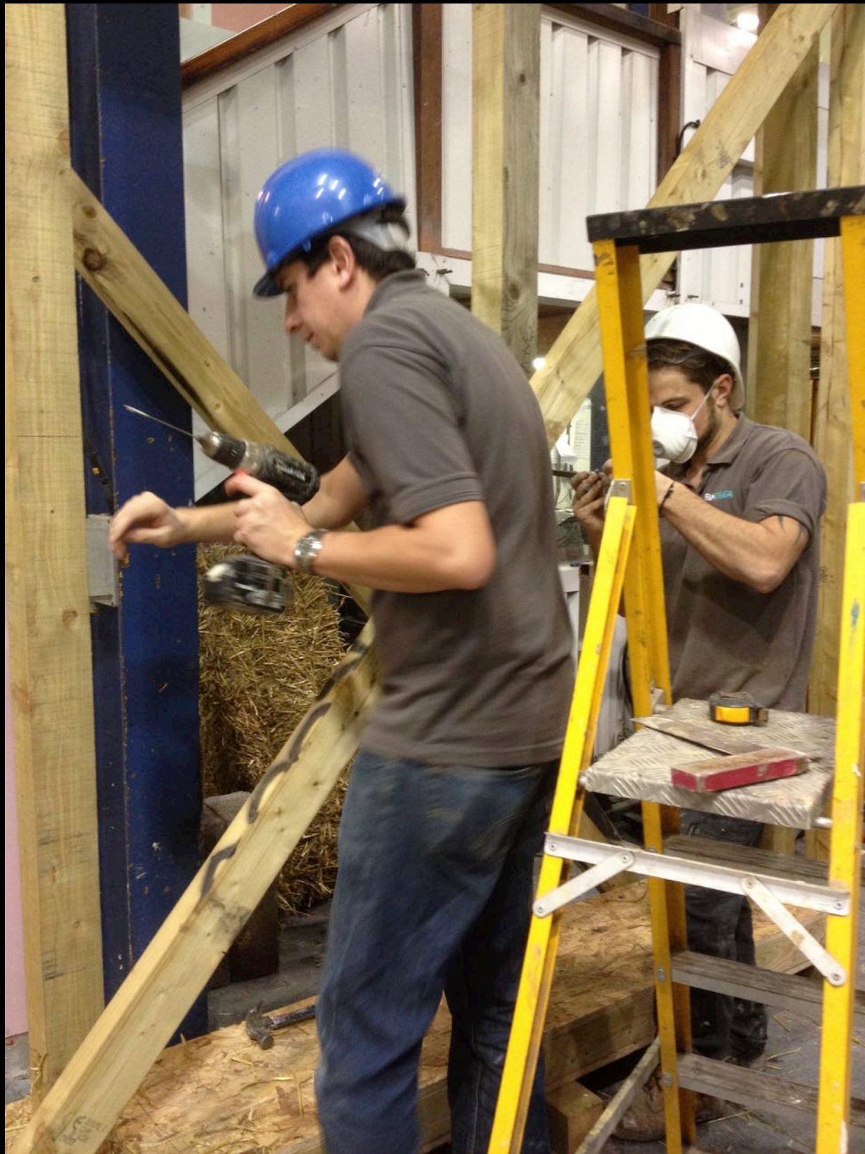
Placing of heat sensors on the posts, the faces of which were set back from the exposed face by 175mm
