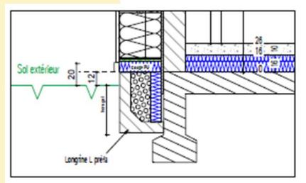
Psi = 0.25 W/m.K Heating demand : 11 kWh/m<sup>2</sup>
